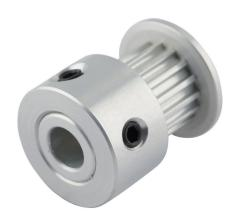
Sung-II Machinery timing pulley, aluminum, 0.08in MXL pitch, 16 tooth, 0.407in pitch diameter, 3/16in bore, oversize hub with flange. For use with 1/4in wide belt.
