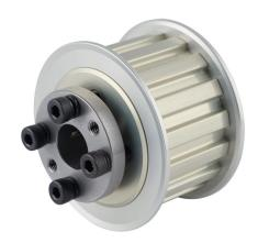
Sung-II Machinery timing pulley, aluminum, 3/8in L pitch, 16 tooth, 1.91in pitch diameter, 1/2in bore, no hub with flanges. For use with 1in wide belt. QD bushing included.
