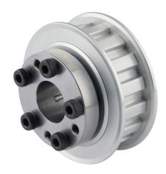
Sung-II Machinery timing pulley, aluminum, 3/8in L pitch, 16 tooth, 1.91in pitch diameter, 5/8in bore, no hub with flanges. For use with 1/2in wide belt. QD bushing included.
