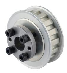
Sung-II Machinery timing pulley, aluminum, 3/8in L pitch, 16 tooth, 1.91in pitch diameter, 1/2in bore, no hub with flanges. For use with 1/2in wide belt. QD bushing included.
