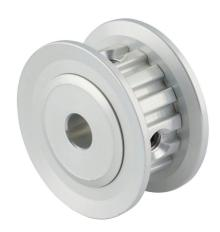
Sung-Il Machinery timing pulley, aluminum, 1/5in XL pitch, 15 tooth, 0.955in pitch diameter, 1/4in bore, no hub with flanges. For use with 3/8in wide belt.
