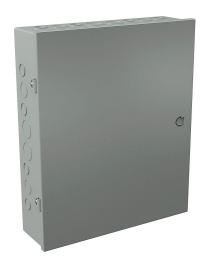
Wiegmann enclosure, NEMA 1, 18 x 15 x 4in (HxWxD), wall mount, with knockouts, carbon steel, ANSI 61 gray, powder coat finish, single-door, integral snap-tight latch.
