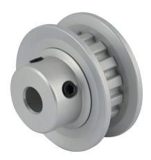
Sung-Il Machinery timing pulley, aluminum, 1/5in XL pitch, 15 tooth, 0.955in pitch diameter, 1/4in bore, hub with flanges. For use with 1/4in wide belt.
