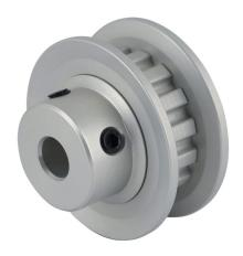
Sung-II Machinery timing pulley, aluminum, 1/5in XL pitch, 15 tooth, 0.955in pitch diameter, 1/4in bore, hub with flanges. For use with 1/4in wide belt.
