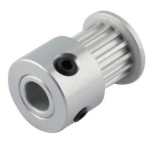
Sung-Il Machinery timing pulley, aluminum, 0.08in MXL pitch, 15 tooth, 0.382in pitch diameter, 3/16in bore, oversize hub with flange. For use with 1/4in wide belt.
