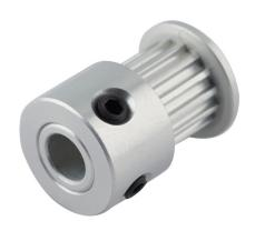
Sung-II Machinery timing pulley, aluminum, 0.08in MXL pitch, 15 tooth, 0.382in pitch diameter, 3/16in bore, oversize hub with flange. For use with 1/4in wide belt.
