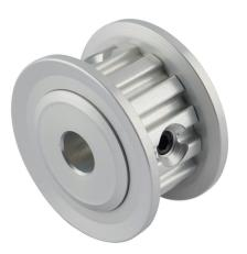
Sung-Il Machinery timing pulley, aluminum, 1/5in XL pitch, 14 tooth, 0.891in pitch diameter, 1/4in bore, no hub with flanges. For use with 3/8in wide belt.
