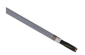
LUTZE SUPERFLEX continuous flexing control cable, shielded, 18 conductors (includes ground), 21 AWG (0.50mm2), bare copper, TPE conductor insulation material, black with white numbers and green/yellow ground, PVC jacket, gray, cut to length.
