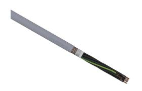
LUTZE SUPERFLEX continuous flexing control cable, shielded, 12 conductors (includes ground), 21 AWG (0.50mm2), bare copper, TPE conductor insulation material, black with white numbers and green/yellow ground, PVC jacket, gray, cut to length.
