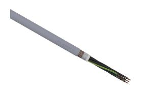
LUTZE SUPERFLEX continuous flexing control cable, shielded, 7 conductors (includes ground), 21 AWG (0.50mm2), bare copper, TPE conductor insulation material, black with white numbers and green/yellow ground, PVC jacket, gray, cut to length.
