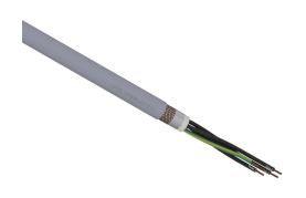
LUTZE SUPERFLEX continuous flexing control cable, shielded, 5 conductors (includes ground), 21 AWG (0.50mm2), bare copper, TPE conductor insulation material, black with white numbers and green/yellow ground, PVC jacket, gray, cut to length.
