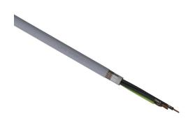
LUTZE SUPERFLEX continuous flexing control cable, shielded, 4 conductors (includes ground), 21 AWG (0.50mm2), bare copper, TPE conductor insulation material, black with white numbers and green/yellow ground, PVC jacket, gray, cut to length.
