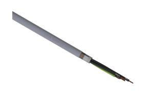
LUTZE SUPERFLEX continuous flexing control cable, shielded, 4 conductors (includes ground), 21 AWG (0.50mm2), bare copper, TPE conductor insulation material, black with white numbers and green/yellow ground, PVC jacket, gray, cut to length.
