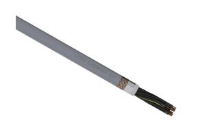
LUTZE SUPERFLEX continuous flexing control cable, shielded, 18 conductors (includes ground), 18 AWG (1.0mm2), bare copper, TPE conductor insulation material, black with white numbers and green/yellow ground, PVC jacket, gray, cut to length.
