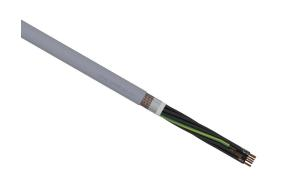
LUTZE SUPERFLEX continuous flexing control cable, shielded, 12 conductors (includes ground), 18 AWG (1.0mm2), bare copper, TPE conductor insulation material, black with white numbers and green/yellow ground, PVC jacket, gray, cut to length.
