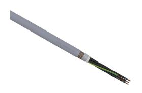
LUTZE SUPERFLEX continuous flexing control cable, shielded, 7 conductors (includes ground), 18 AWG (1.0mm2), bare copper, TPE conductor insulation material, black with white numbers and green/yellow ground, PVC jacket, gray, cut to length.
