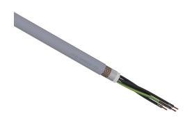
LUTZE SUPERFLEX continuous flexing control cable, shielded, 5 conductors (includes ground), 18 AWG (1.0mm2), bare copper, TPE conductor insulation material, black with white numbers and green/yellow ground, PVC jacket, gray, cut to length.
