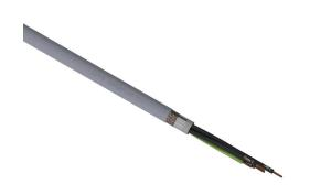
LUTZE SUPERFLEX continuous flexing control cable, shielded, 4 conductors (includes ground), 18 AWG (1.0mm2), bare copper, TPE conductor insulation material, black with white numbers and green/yellow ground, PVC jacket, gray, cut to length.
