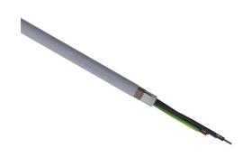
LUTZE SUPERFLEX continuous flexing control cable, shielded, 3 conductors (includes ground), 18 AWG (1.0mm2), bare copper, TPE conductor insulation material, black with white numbers and green/yellow ground, PVC jacket, gray, cut to length.
