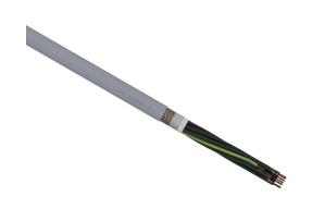
LUTZE SUPERFLEX continuous flexing control cable, shielded, 12 conductors (includes ground), 16 AWG (1.50mm2), bare copper, TPE conductor insulation material, black with white numbers and green/yellow ground, PVC jacket, gray, cut to length.
