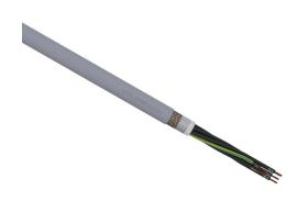
LUTZE SUPERFLEX continuous flexing control cable, shielded, 7 conductors (includes ground), 16 AWG (1.50mm2), bare copper, TPE conductor insulation material, black with white numbers and green/yellow ground, PVC jacket, gray, cut to length.
