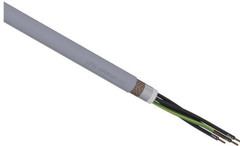
LUTZE SUPERFLEX continuous flexing control cable, shielded, 5 conductors (includes ground), 16 AWG (1.50mm<sup>2</sup>), bare copper, TPE conductor insulation material, black with white numbers and green/yellow ground, PVC jacket, gray, cut to length.
