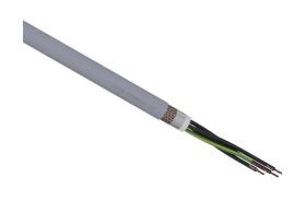
LUTZE SUPERFLEX continuous flexing control cable, shielded, 5 conductors (includes ground), 16 AWG (1.50mm2), bare copper, TPE conductor insulation material, black with white numbers and green/yellow ground, PVC jacket, gray, cut to length.
