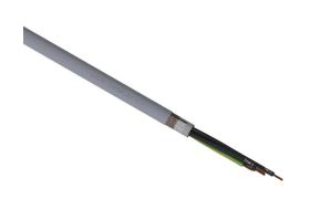
LUTZE SUPERFLEX continuous flexing control cable, shielded, 4 conductors (includes ground), 16 AWG (1.50mm2), bare copper, TPE conductor insulation material, black with white numbers and green/yellow ground, PVC jacket, gray, cut to length.
