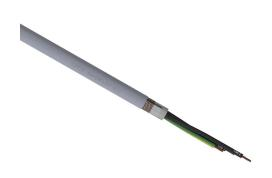
LUTZE SUPERFLEX continuous flexing control cable, shielded, 3 conductors (includes ground), 16 AWG (1.50mm2), bare copper, TPE conductor insulation material, black with white numbers and green/yellow ground, PVC jacket, gray, cut to length.
