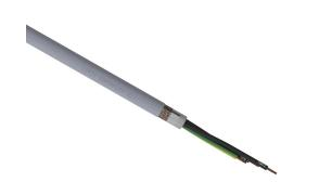
LUTZE SUPERFLEX continuous flexing control cable, shielded, 3 conductors (includes ground), 16 AWG (1.50mm2), bare copper, TPE conductor insulation material, black with white numbers and green/yellow ground, PVC jacket, gray, cut to length.
