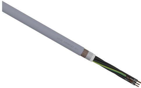
LUTZE SUPERFLEX continuous flexing control cable, shielded, 7 conductors (includes ground), 14 AWG (2.50mm<sup>2</sup>), bare copper, TPE conductor insulation material, black with white numbers and green/yellow ground, PVC jacket, gray, cut to length.
