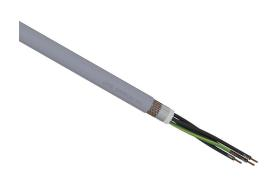
LUTZE SUPERFLEX continuous flexing control cable, shielded, 5 conductors (includes ground), 14 AWG (2.50mm2), bare copper, TPE conductor insulation material, black with white numbers and green/yellow ground, PVC jacket, gray, cut to length.
