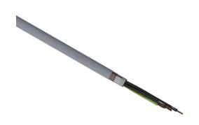
LUTZE SUPERFLEX continuous flexing control cable, shielded, 4 conductors (includes ground), 14 AWG (2.50mm2), bare copper, TPE conductor insulation material, black with white numbers and green/yellow ground, PVC jacket, gray, cut to length.
