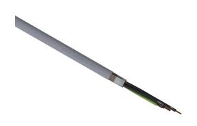
LUTZE SUPERFLEX continuous flexing control cable, shielded, 4 conductors (includes ground), 12 AWG (4.0mm2), bare copper, TPE conductor insulation material, black with white numbers and green/yellow ground, PVC jacket, gray, cut to length.
