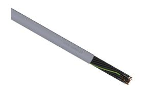
LUTZE SUPERFLEX continuous flexing control cable, unshielded, 25 conductors (includes ground), 21 AWG (0.50mm2), bare copper, TPE conductor insulation material, black with white numbers and green/yellow ground, PVC jacket, gray, cut to length.
