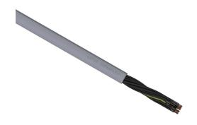
LUTZE SUPERFLEX continuous flexing control cable, unshielded, 18 conductors (includes ground), 21 AWG (0.50mm2), bare copper, TPE conductor insulation material, black with white numbers and green/yellow ground, PVC jacket, gray, cut to length.
