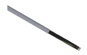
LUTZE SUPERFLEX continuous flexing control cable, unshielded, 12 conductors (includes ground), 21 AWG (0.50mm2), bare copper, TPE conductor insulation material, black with white numbers and green/yellow ground, PVC jacket, gray, cut to length.
