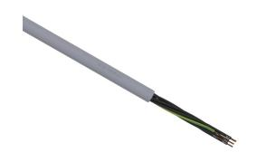
LUTZE SUPERFLEX continuous flexing control cable, unshielded, 7 conductors (includes ground), 21 AWG (0.50mm2), bare copper, TPE conductor insulation material, black with white numbers and green/yellow ground, PVC jacket, gray, cut to length.
