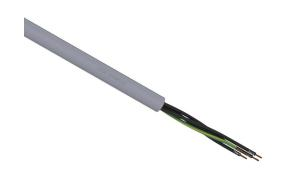
LUTZE SUPERFLEX continuous flexing control cable, unshielded, 5 conductors (includes ground), 21 AWG (0.50mm2), bare copper, TPE conductor insulation material, black with white numbers and green/yellow ground, PVC jacket, gray, cut to length.
