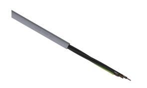
LUTZE SUPERFLEX continuous flexing control cable, unshielded, 4 conductors (includes ground), 21 AWG (0.50mm2), bare copper, TPE conductor insulation material, black with white numbers and green/yellow ground, PVC jacket, gray, cut to length.
