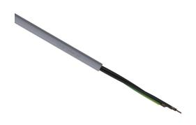
LUTZE SUPERFLEX continuous flexing control cable, unshielded, 3 conductors (includes ground), 21 AWG (0.50mm2), bare copper, TPE conductor insulation material, black with white numbers and green/yellow ground, PVC jacket, gray, cut to length.
