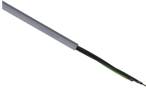
LUTZE SUPERFLEX continuous flexing control cable, unshielded, 3 conductors (includes ground), 21 AWG (0.50mm<sup>2</sup>), bare copper, TPE conductor insulation material, black with white numbers and green/yellow ground, PVC jacket, gray, cut to length.
