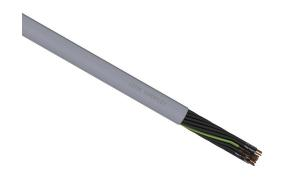
LUTZE SUPERFLEX continuous flexing control cable, unshielded, 34 conductors (includes ground), 18 AWG (1.0mm2), bare copper, TPE conductor insulation material, black with white numbers and green/yellow ground, PVC jacket, gray, cut to length.
