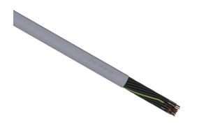
LUTZE SUPERFLEX continuous flexing control cable, unshielded, 25 conductors (includes ground), 18 AWG (1.0mm2), bare copper, TPE conductor insulation material, black with white numbers and green/yellow ground, PVC jacket, gray, cut to length.
