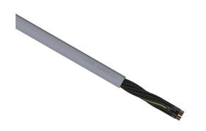
LUTZE SUPERFLEX continuous flexing control cable, unshielded, 18 conductors (includes ground), 18 AWG (1.0mm2), bare copper, TPE conductor insulation material, black with white numbers and green/yellow ground, PVC jacket, gray, cut to length.
