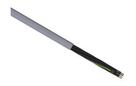
LUTZE SUPERFLEX continuous flexing control cable, unshielded, 12 conductors (includes ground), 18 AWG (1.0mm2), bare copper, TPE conductor insulation material, black with white numbers and green/yellow ground, PVC jacket, gray, cut to length.
