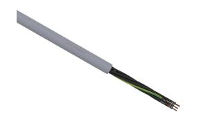
LUTZE SUPERFLEX continuous flexing control cable, unshielded, 7 conductors (includes ground), 18 AWG (1.0mm2), bare copper, TPE conductor insulation material, black with white numbers and green/yellow ground, PVC jacket, gray, cut to length.
