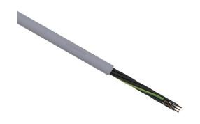
LUTZE SUPERFLEX continuous flexing control cable, unshielded, 7 conductors (includes ground), 18 AWG (1.0mm2), bare copper, TPE conductor insulation material, black with white numbers and green/yellow ground, PVC jacket, gray, cut to length.
