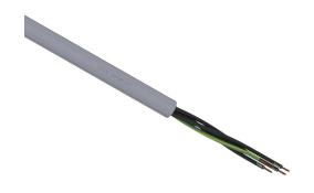
LUTZE SUPERFLEX continuous flexing control cable, unshielded, 5 conductors (includes ground), 18 AWG (1.0mm2), bare copper, TPE conductor insulation material, black with white numbers and green/yellow ground, PVC jacket, gray, cut to length.
