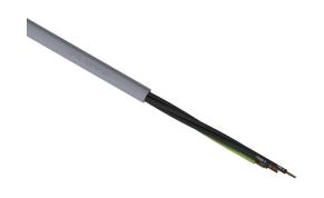
LUTZE SUPERFLEX continuous flexing control cable, unshielded, 4 conductors (includes ground), 18 AWG (1.0mm2), bare copper, TPE conductor insulation material, black with white numbers and green/yellow ground, PVC jacket, gray, cut to length.
