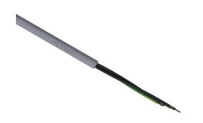
LUTZE SUPERFLEX continuous flexing control cable, unshielded, 3 conductors (includes ground), 18 AWG (1.0mm2), bare copper, TPE conductor insulation material, black with white numbers and green/yellow ground, PVC jacket, gray, cut to length.
