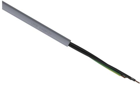
LUTZE SUPERFLEX continuous flexing control cable, unshielded, 3 conductors (includes ground), 18 AWG (1.0mm<sup>2</sup>), bare copper, TPE conductor insulation material, black with white numbers and green/yellow ground, PVC jacket, gray, cut to length.
