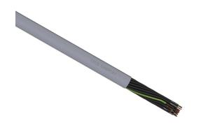
LUTZE SUPERFLEX continuous flexing control cable, unshielded, 25 conductors (includes ground), 16 AWG (1.50mm2), bare copper, TPE conductor insulation material, black with white numbers and green/yellow ground, PVC jacket, gray, cut to length.
