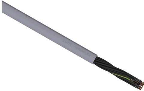
LUTZE SUPERFLEX continuous flexing control cable, unshielded, 18 conductors (includes ground), 16 AWG (1.50mm<sup>2</sup>), bare copper, TPE conductor insulation material, black with white numbers and green/yellow ground, PVC jacket, gray, cut to length.
