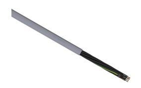
LUTZE SUPERFLEX continuous flexing control cable, unshielded, 12 conductors (includes ground), 16 AWG (1.50mm2), bare copper, TPE conductor insulation material, black with white numbers and green/yellow ground, PVC jacket, gray, cut to length.
