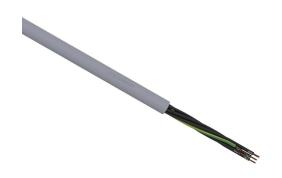
LUTZE SUPERFLEX continuous flexing control cable, unshielded, 7 conductors (includes ground), 16 AWG (1.50mm2), bare copper, TPE conductor insulation material, black with white numbers and green/yellow ground, PVC jacket, gray, cut to length.
