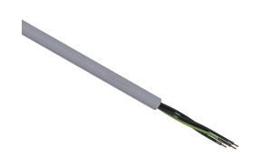
LUTZE SUPERFLEX continuous flexing control cable, unshielded, 5 conductors (includes ground), 16 AWG (1.50mm2), bare copper, TPE conductor insulation material, black with white numbers and green/yellow ground, PVC jacket, gray, cut to length.
