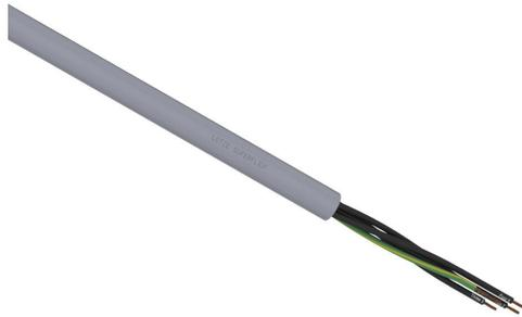
LUTZE SUPERFLEX continuous flexing control cable, unshielded, 5 conductors (includes ground), 16 AWG (1.50mm<sup>2</sup>), bare copper, TPE conductor insulation material, black with white numbers and green/yellow ground, PVC jacket, gray, cut to length.
