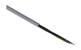
LUTZE SUPERFLEX continuous flexing control cable, unshielded, 4 conductors (includes ground), 16 AWG (1.50mm2), bare copper, TPE conductor insulation material, black with white numbers and green/yellow ground, PVC jacket, gray, cut to length.
